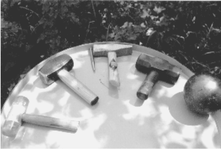
Fig. B.10 A collection of hammers used by tuner Lawrence Mayers. Left to right: Small tuning/smoothing hammer, large tuning hammer, punch together with grooving hammer (also used for tuning of the smallest notes), backing hammer and shot-put. Photograph by Linus Torell.
