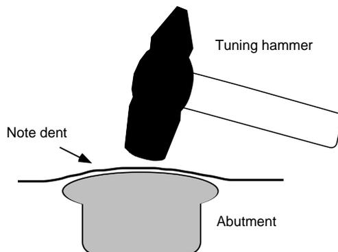
Fig. 17.3 Using an abutment to shape a note.
