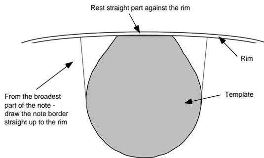
Fig. 17.2 Shape of a suggested template for an outer note.
