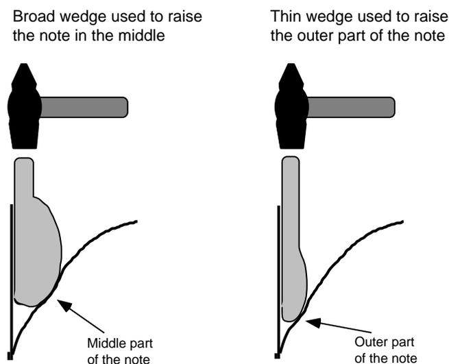
Fig. 17.1 Using wedges to raise outer notes.
