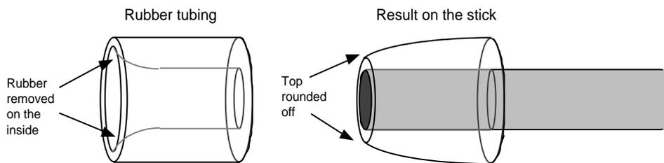
Fig. 16.4 Tenor stick with rounded top.
